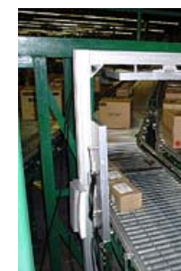
An RFID scanner at a W
